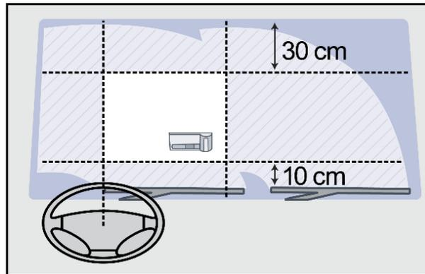
Figure 21: the correct installation of the GO-Box
