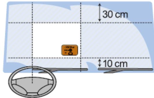
Figure 22: the correct installation of the GO-Box
